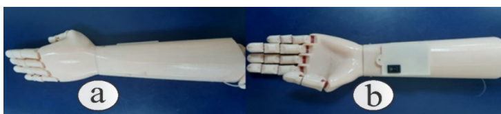
Figure 9 – Design of the prosthesis in 3D printing, a) Upper part of the prosthesis, b) Lower part of the prosthesis.
