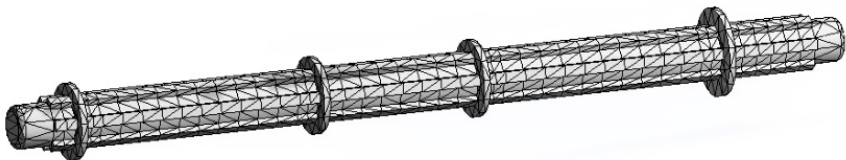
Figure 6 – Meshing of the transmission axis of movement.
