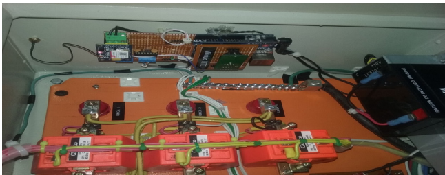
Figure 7 – Central Processing Node
